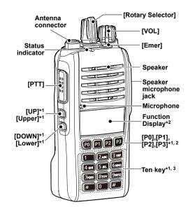
\*1: The key functions are dealer assignable. \*2: Only for the Simple key and Ten-key types. \*3: Only for the Ten-key type.
