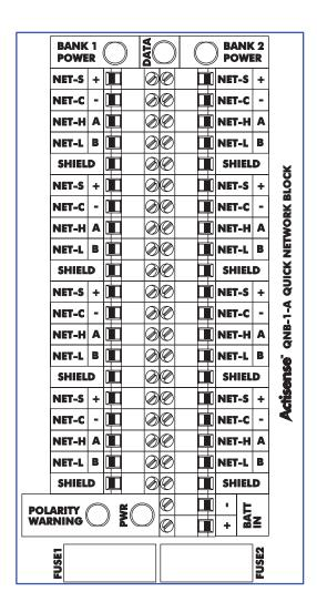
The board is clearly labelled with the functions of each connector and indicator. A detailed description of each label is as follows:
